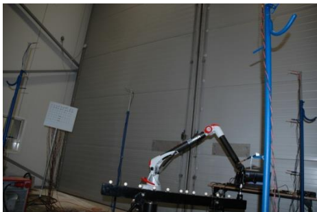
Fig. 1. 7-axes AACMM placed in the so-called „temperature cage“
