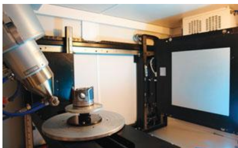
Fig. 1. Industrial CT Nikon XT H 225 https://www.nikonmetrology.com/en-gb/product/xt-h-225
