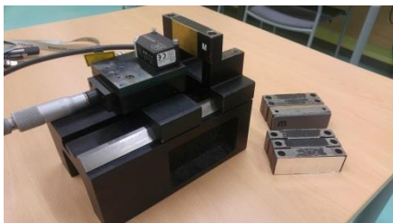
Fig. 1. Determination of statistical metrological properties of laser heads
